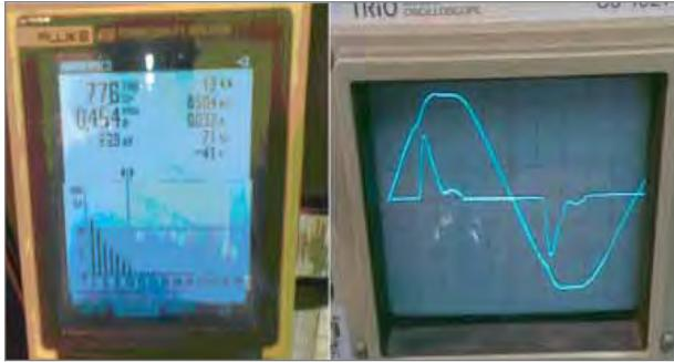
Figures 12 and 13: four CFLs in parallel
